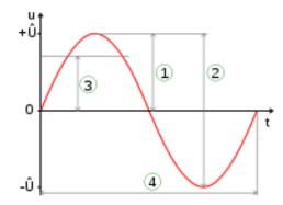
Description : A sinodial voltage. 1 = Amplitude (peak), 2 = Peak-to-peak, 3 = RMS, 4 = Wave period
